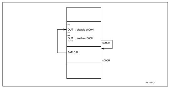
The branch prediction mechanism of the embedded Pentium processor, however, predicts that the RET instruction is going to transfer control to the segment at address C000H and performs a prefetch from that address prior to the OUT instruction that re-enables that memory address. The result is that no BRDY is returned for that prefetch cycle and the system hangs.
